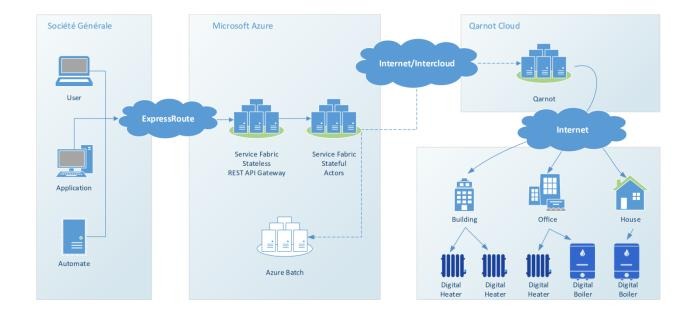
High-performance financial calculations are broken into discrete jobs and tasks by Service Fabric, then distributed to available cloud computing environments.
